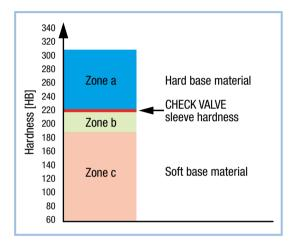
Zone a - Hard base material (HB > 220) To achieve the allowable working pressure, anchorage to the bore roughness of the base material is required. Roughness  $R_z = 10-30 \mu m$ .
