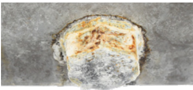
HA-SCHRAUBENGARNITUREN® from ESKA® vs. HV-bolt-set according to DIN EN 14399-1 after 1008 hours of salt spray test (screwed in aluminium)
