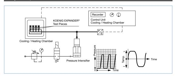
The KOENIG EXPANDER® is subjected to a pressure cycling test under varying environmental conditions. The test determines the levels of pressure that can be absorbed by the part by applying intermittent pressure loads and temperature fluctuations to confirm the sealing plug is not squeezed out.
