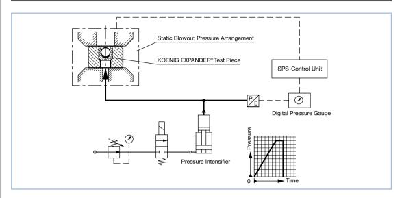
The KOENIG EXPANDER® is statically loaded up to burst pressure. This test is performed at SFC KOENIG for functional testing during the production process.
