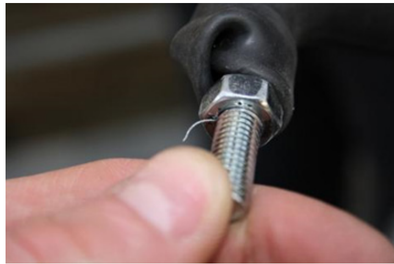
Figure 2: Burr on thread
