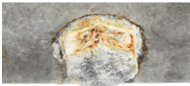
HA-SCHRAUBENGARNITUREN® from ESKA® vs. HV-bolt-set according to DIN EN 14399-1 after 1008 hours of salt spray test (screwed in aluminium)
