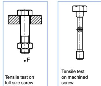
Tensile strength at rupture in cylindrical shank:
