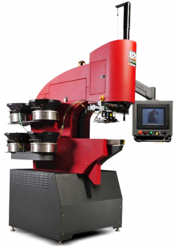
The Haeger® 824 OneTouch 4e self-clinching system with 4-way automatic feed system
