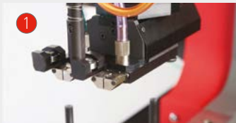
FROM STATION 1 TO STATION 2 – DEPOSITING THE UPPER TOOL
