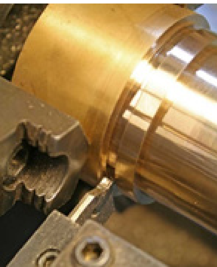
Figure 4: Machining of bronze
