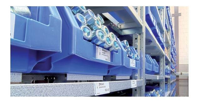
This unique, fully automated system with sensor monitoring is ideal for supermarket areas and line assembly. SmartBin manages anything from small parts weighing just a few grams to large parts of up to 1,000 kg per palette. Weight sensors ensure continuous online inventory monitoring. Orders are triggered automatically and enable a seamless supply.
