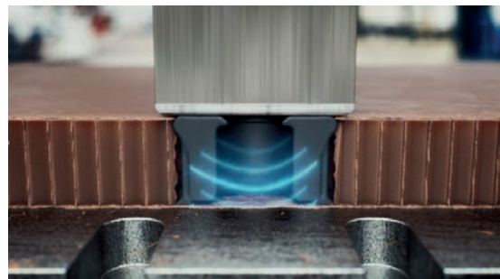
Apply MM-Welding process using ultrasonic energy to liquify the polymer and create a connection to both layers.
