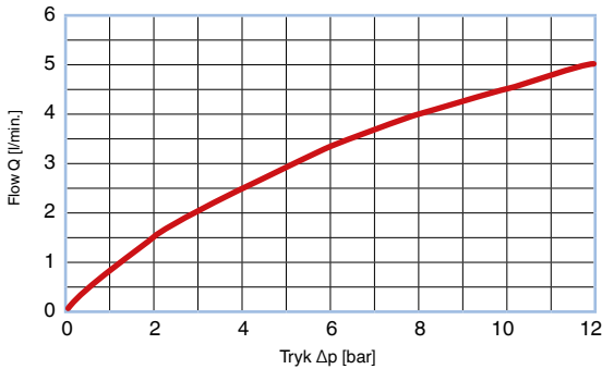
CHECK VALVE® Flowkurve – unscreened BFAA055U014; T = 50 °C, hydraulikolie HLP46
