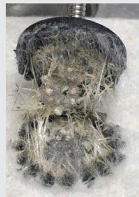
Pull-out test shows intensive integration into substrate material.
