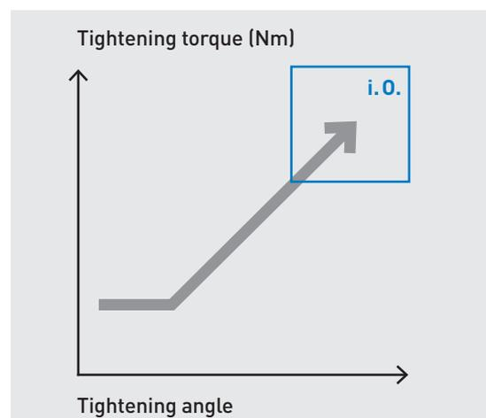
**Illustration 1** Correct at the first go mounted - the right assembly window for a reliable connection. (Illustration from brochure Tribological dry coatings, page 3)
