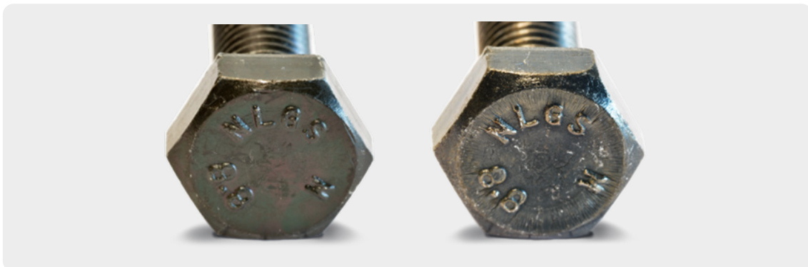
Comparing zinc-plated black chromate containing hexavalent chromium on the left and black passivate that is free from hexavalent chromium on the right.
