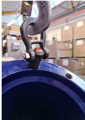
The threaded lifting pin can be inserted into the thread of the cast iron blank at the push of a button.
