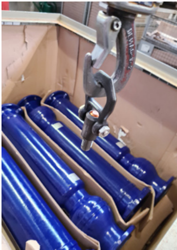
Thanks to the movable shackle, the threaded lifting pin can be easily attached to the crane hook.
