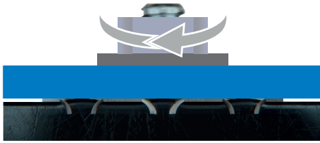
InWVerse® Fastener tightened to 2 Nm
