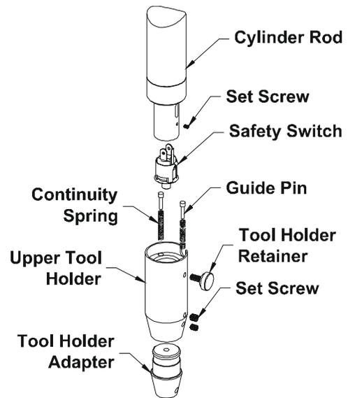
**Figure 4.1:** The Safety Switch is inside the Upper Tool Holder.
