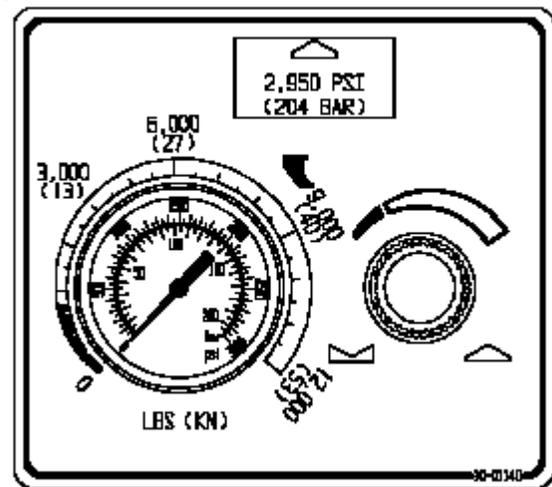
**Figure 4.8:** Turn the Force Adjust knob on the Control Panel to 3,000 lb/13 kN.
