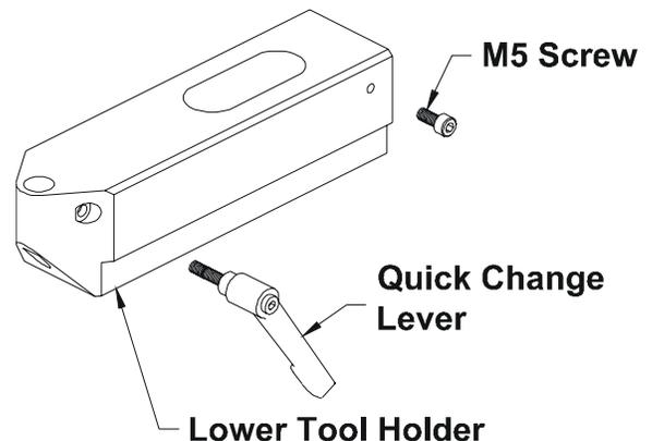
**Figure 3.8:** The Quick Change Lever makes it easy to change lower tools.
