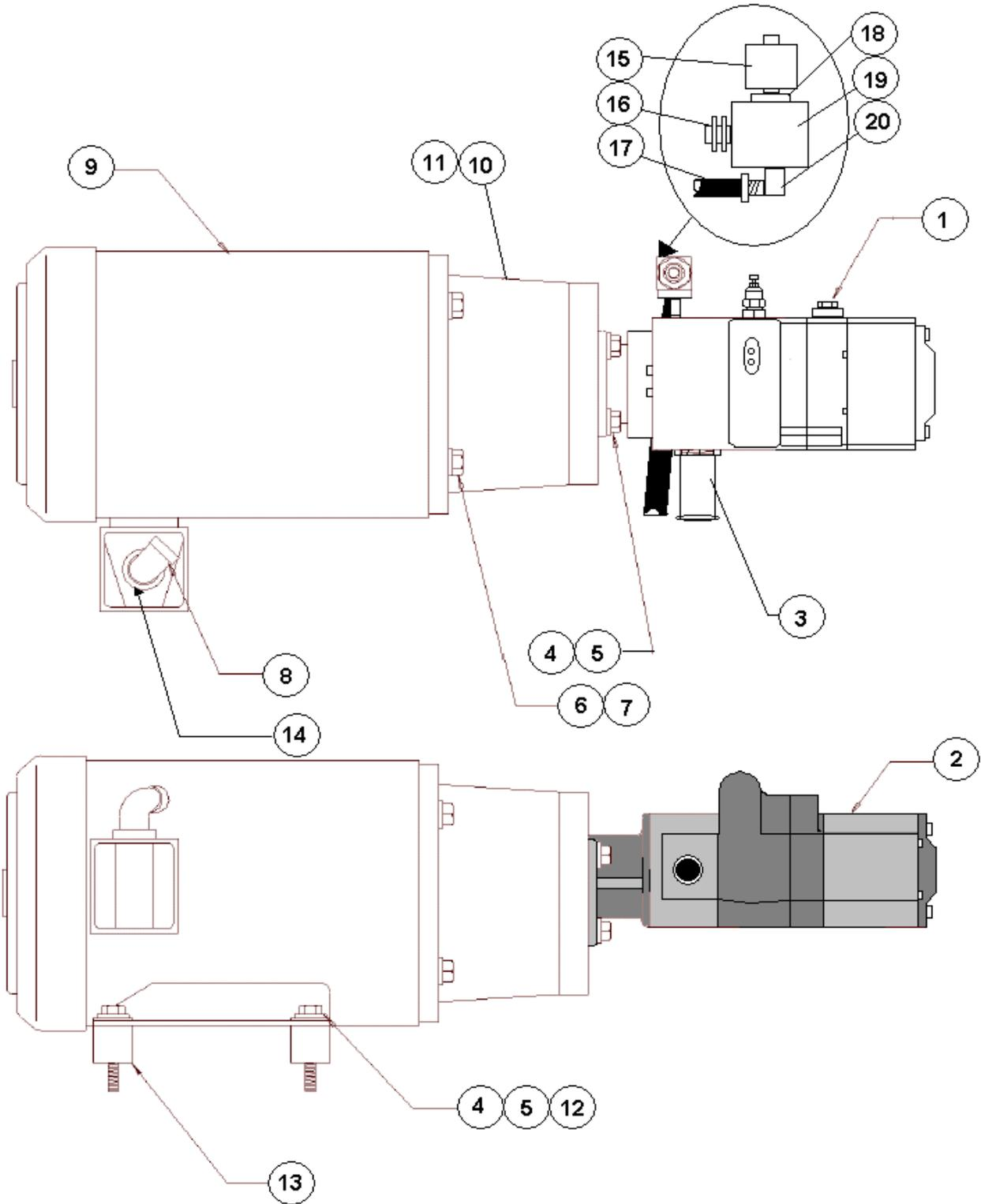
Hardware Insertion MachineMotor Pump Assembly
