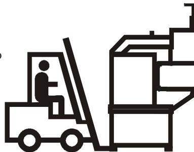
Always position the forklift to the rear of the machine.
