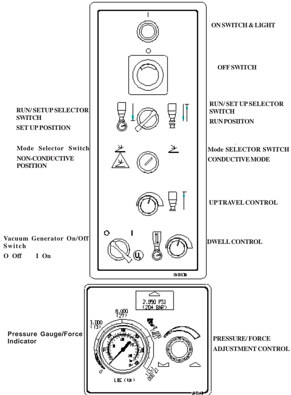
**Figure 5.2:** These Control Panels contain most of the controls needed to operate the machine.
