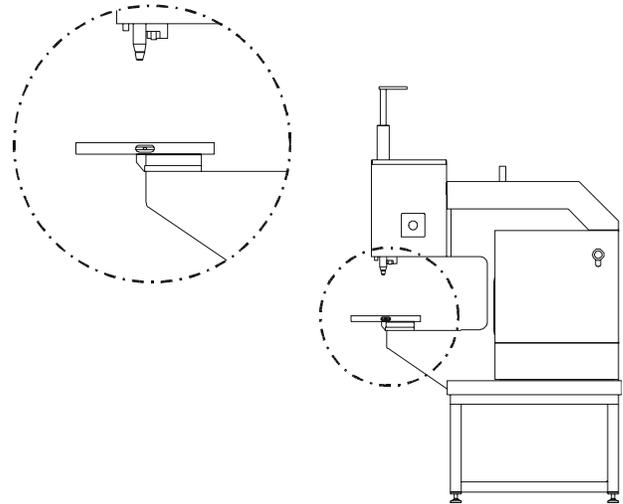
**Figure 3.1:** Level the machine by using the Lower Tool Holder as a reference surface
