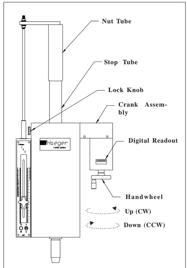
**Figure 5.9:** The Digital Readout Option for the Positive Stop System makes setup of the Positive Stop System easier.
