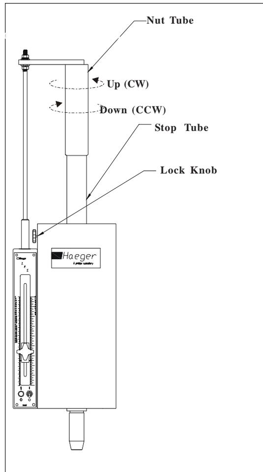
**Figure 5.9:** The Positive Stop System helps stop the machine cylinder at the same place every time.
