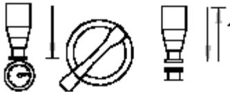
**Figure 4.5:** Turn the Run/Setup Switch to the Run position.
