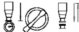
**Figure 4.9:** Turn the Run/Setup Switch in the Run position.
