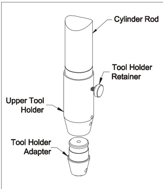
**Figure 3.7:** The Upper Tool Holder comes installed in your Hardware Insertion Machine.
