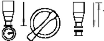
**Figure 4.5:** Turn the Run/Setup Switch to the Run position.
