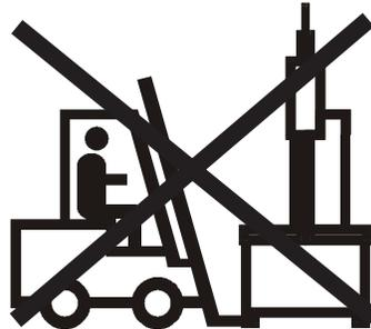
Never lift with the forklift in front or on the side.
