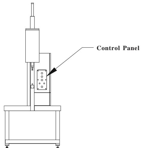
**Figure 4.3:** The Control Panel is on the front side of the Main Electrical Control Cabinet.
