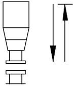
The Run Mode position on the selector switch is on the right and is represented by this symbol.
