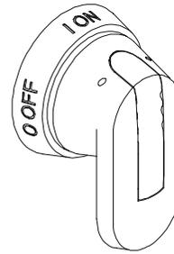
**Figure 3.5:** Turn the machine's Main Disconnect Switch to the On position.
