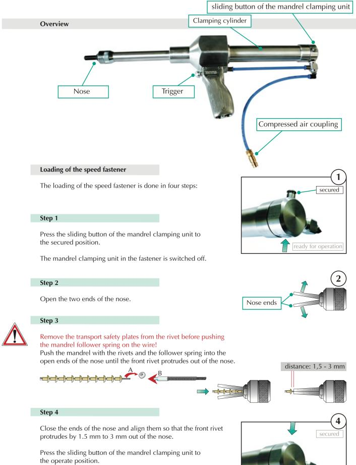
The mandrel clamping unit is switched on.
