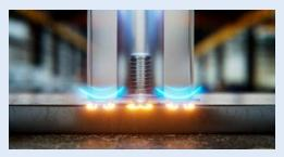
Ultrasonic energy is applied. Within a second the localized thermoplastic melting generates a strong form-locking.
