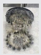
Pull-out test shows intensive integration into substrate material.
