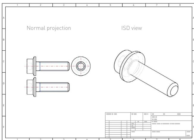
Fig. 4: 2D, e.g. three views with isometric drawing in frame (DIN)
