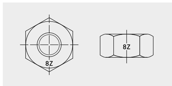
Fig. 17: Example of the marking used on hot dip-galvanized nuts tapped oversize to tolerance position 6AZ after coating
