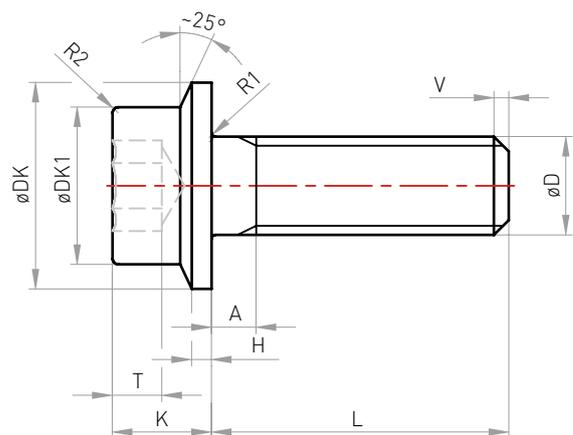
Fig. 5: Dimensioning (e.g. front view)
