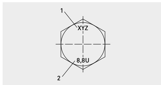
Fig. 16: Example of the marking used on hot dip-galvanized bolts and screws with threads undersized to tolerance class 6az before coating
