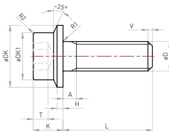
Fig. 5: Dimensioning (e.g. front view)
