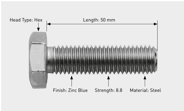
Fig. 1: Hex Cap Screw DIN 933 M10 x 50 mm Property Class 8.8 Zinc Blue
