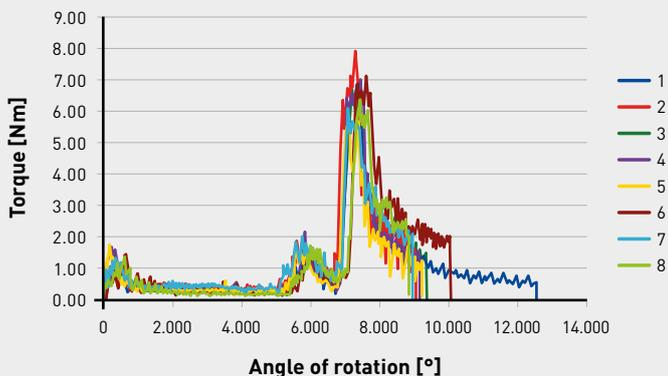
Fig. 13: Technically optimum torque/angle of rotation curves
