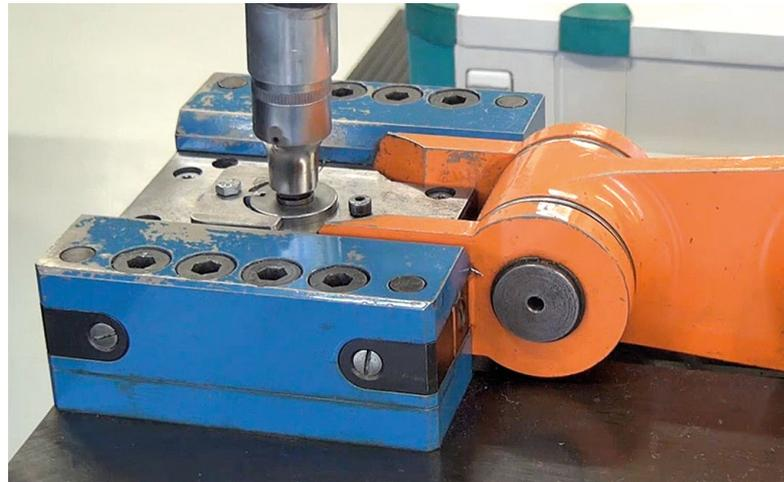
Fig. 15: Junker vibration test
