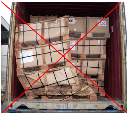
Problem: Weak cask cover and heavy pallets on top / cardboard boxes and pallets without sufficient fixation
