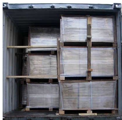
Problem: Weak cask cover and heavy pallets on top / cardboard boxes and pallets without sufficient fixation
