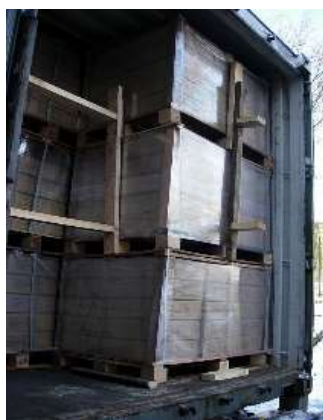
Problem: Weak cask cover and heavy pallets on top / cardboard boxes and pallets without sufficient fixation
