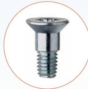
The finished product delivered by Bossard is a specially made screw that has a thread diameter of 4.5 mm. It cuts the thread the first time it is inserted and it comes with a special supporting shank. The Torx® drive prevents damage to the screw head at high torques. The underlying round flange holds the chair parts together securely.
